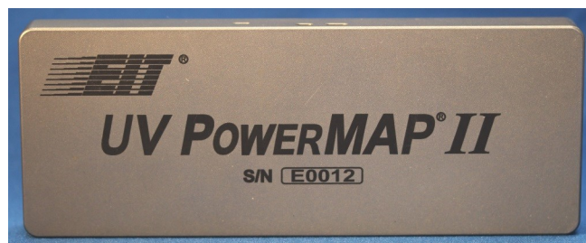
PowerMAP II: Smaller size, larger memory, USB connection, UV & temperature profiles
